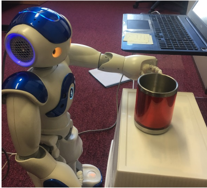
Figure 10: Success execution: The NAO robot can reach the cup
